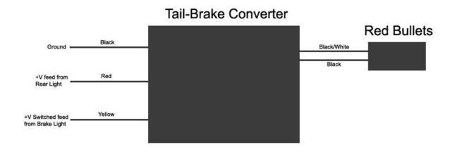
The Yellow, Red and Black wires feeding the converter can all be spliced into your existing tail / brake light wiring. This preserves your current tail / brake light but adds the Red Bullets.
