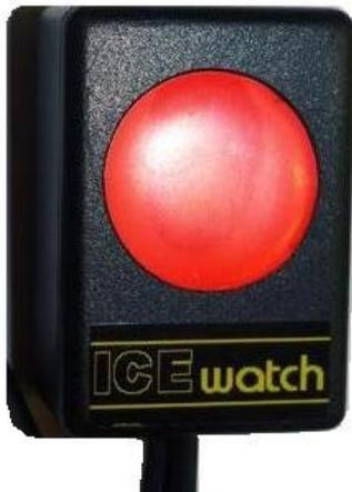
The SMiDSY **ICEwatch** unit continuously monitors the air temperature around your bike, providing you with advance warning of dangerous road conditions.
